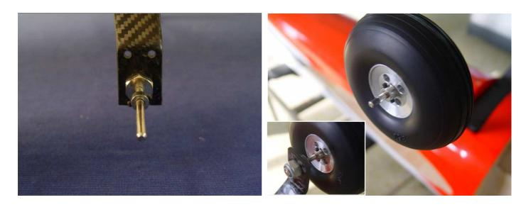
Make the flat sides of the axle bolt vertical with ground. Then tighten the lock nut against the landing gear strut.
