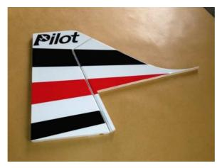
The fin was glued with the rudder in factory.
