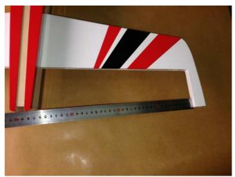
Apply 30-minute epoxy to both the stab and fuselage sections and slide the stab into position.
