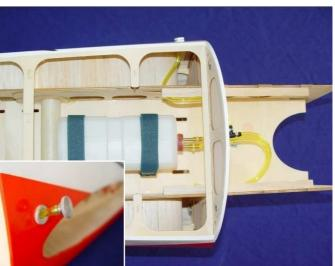
Fule tank and fuel dot have been installed. Just tighten the velcro ties.
