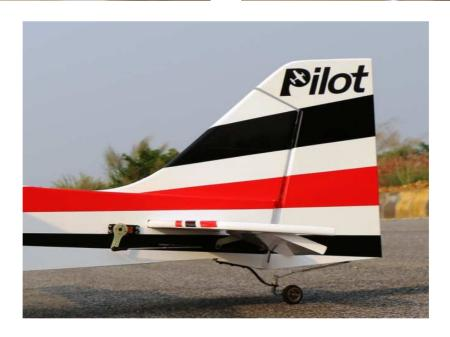
Install the servo arms facing toward the ground and adjust pushrod in proper length to keep the aileron panel on the neutral position as shown.
