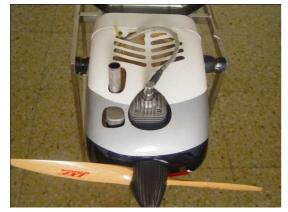
Ensue all the corner are rounded and not sharp 90 degrees against splitting under vibration. Trial fit till the cowl is right
