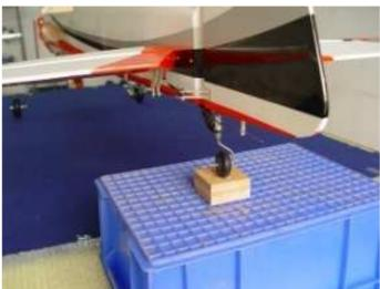
Lift the rear of fuse and line the wheel pant up with the ground by slipping them over the axles and supporting them from the rear for the proper clearance.
