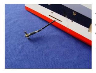
The rudder cables and couplers have been installed.
