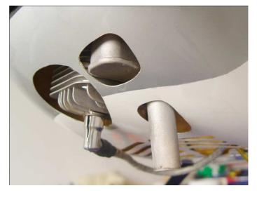
Make or use the supplied pattern of the exit air cooling. But do not cut off the cowing mounting holes position.
