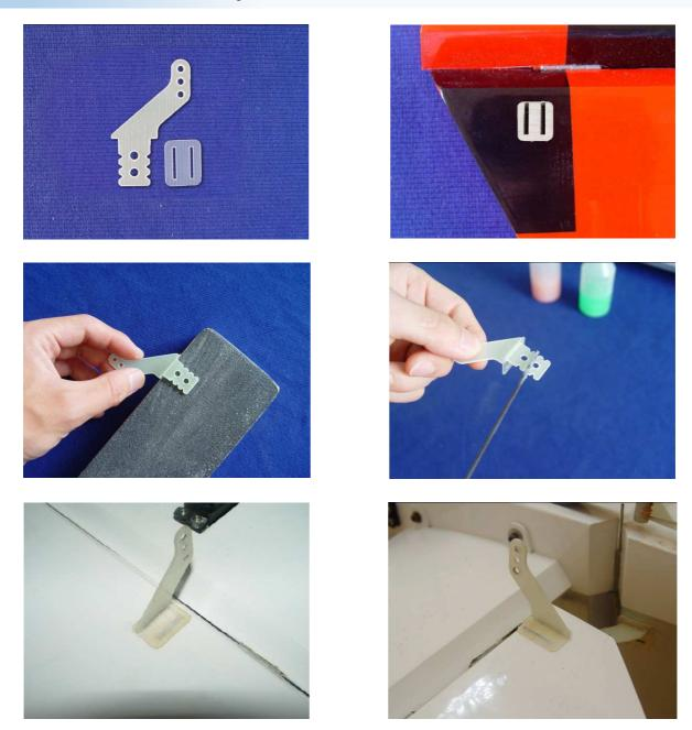
Slice covering over factory installed slots. Press control horn into position. Trace around the locking plate with a knife and remove the covering.
