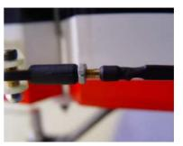
Shrink the heat shrinking tube on the brass tube.
