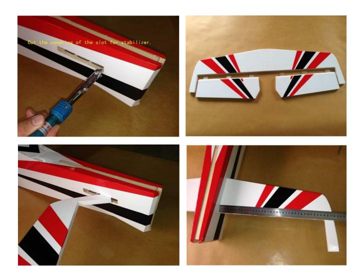
Cut the covering of the slot for stabilizer.
