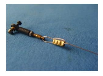
Turn on your radio to keep the servo neutral. Mount the pre-installed boll link to the rudder arm without locking nut. Put two brass tube through the cable and thread through the coupler hole. Ensure the cables are straight.
