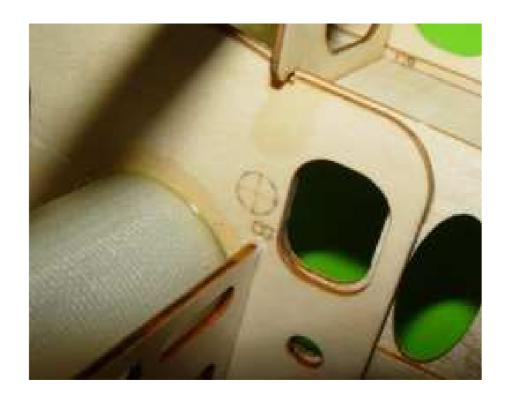
The location of CG has been marked inside of this plane. Usually it's near the wing tube.
