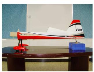
Install the landing gear with the bolts and locking nuts. Note: Don't over tighten and crack the carbon fiber.
