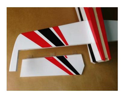
Mix some "30-minute epoxy" and glue one side of the hinge to the elevator.
