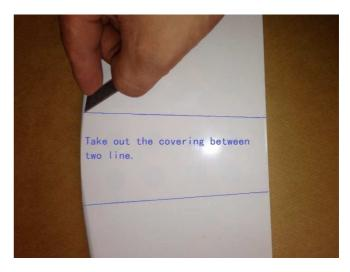
Once the stab is centered, draw a line on both side of the stab as shown, both top and bottom of the stab.
