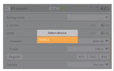
Click the RX to complete the binding after the receiver window pops up, the system will confirm "Bind succeed".
