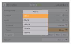
Open the Power menu bar and select the desired power level according to usage.
