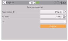
When the "RX Connected" page pops up, press the [REGISTER] to complete the Registration procedure and then power the receiver off.
