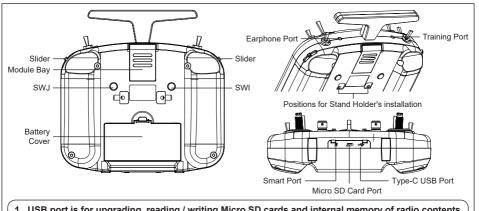
1. USB port is for upgrading, reading / writing Micro SD cards and internal memory of radio contents and charging. (Micro SD card is not provided with shipment.)
