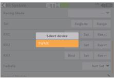
Click the RX to complete the binding after the receiver window pops up, the system will confirm "Bind succeed".
