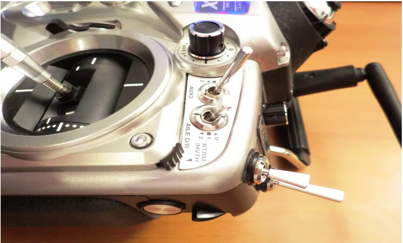
Pos 0 = normal flight with reduced throws (in this case is used the aileron D/R switch)
