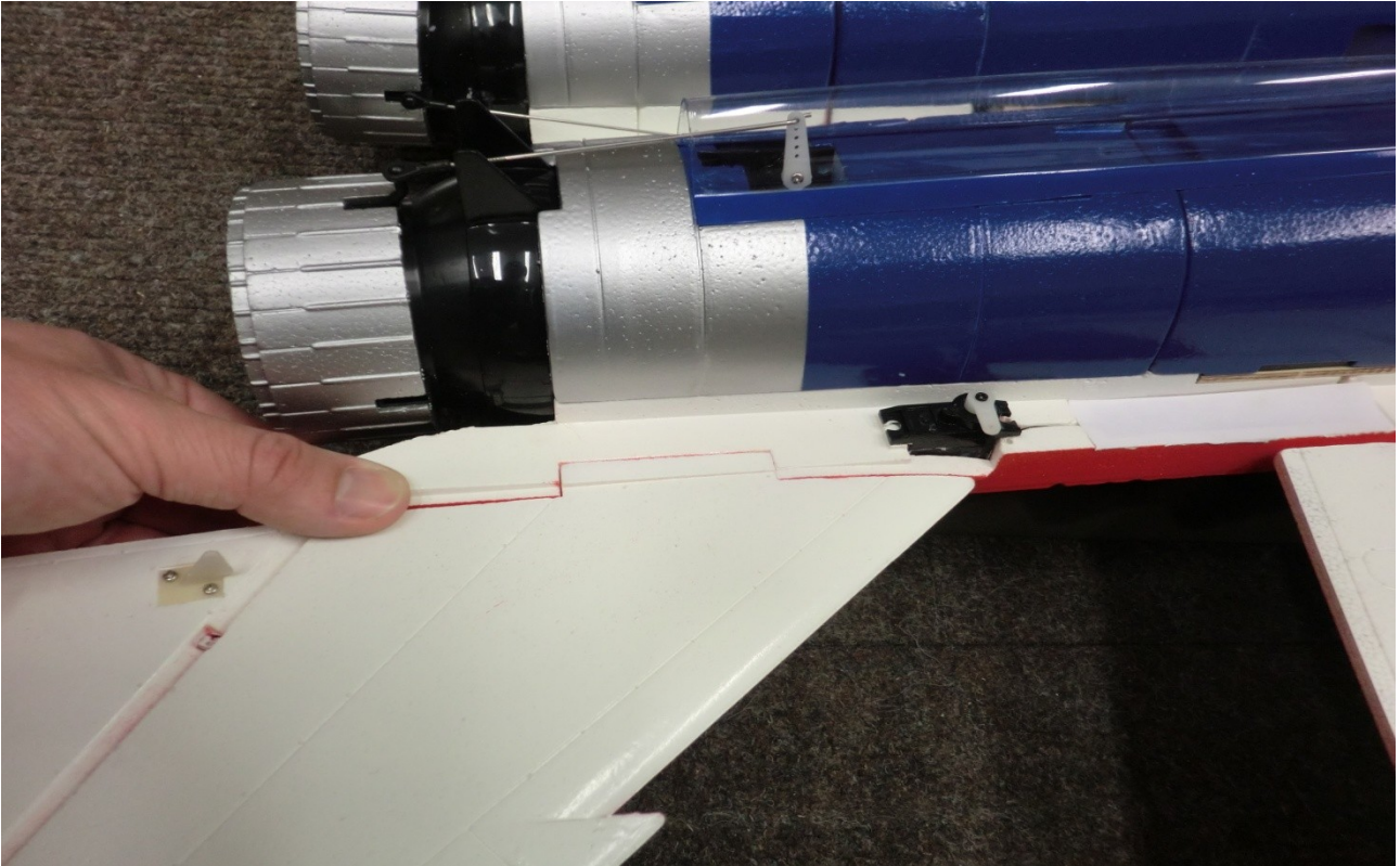
Apply a light coat of 5-minute epoxy on the stabiliser panel.
