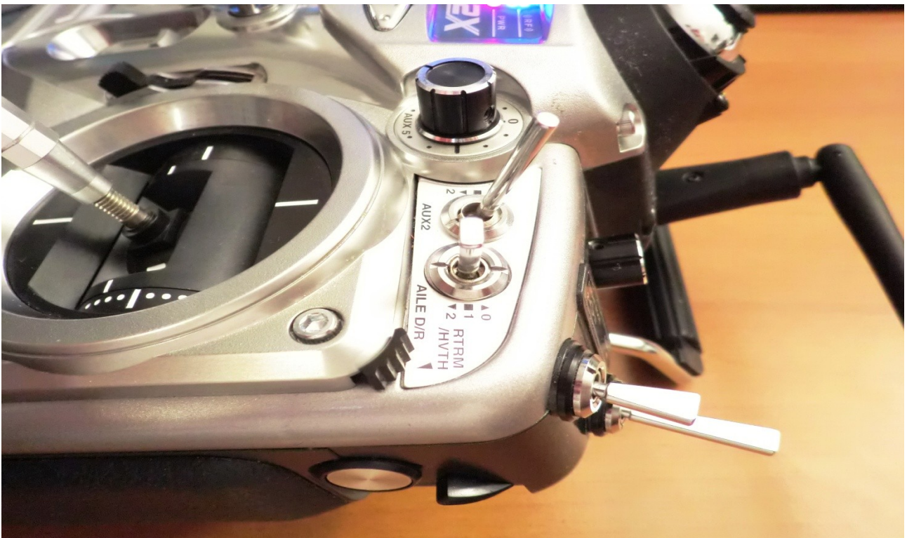
Pos 1 = flight with full rates for start, landing flat spins with GYRO in OFF position (in this case is used the aileron D/R switch)
