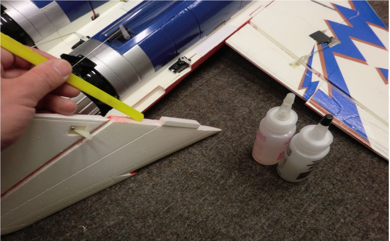
Apply a light coat of 5-minute epoxy on the stabiliser panel.
