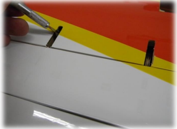
56-) Remove the masking tape. Using your finger, locate the three slots in the wing, in front of the spoilers. Once located, cut the covering to allow the spoilers to move upwards.
